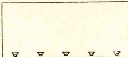
Fig. 4—Side-by-side speakers can create problems unless carefully phased.
